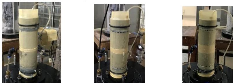
a) 5 mm sand cushion b) 10 mm sand cushion c) 20 mm sand cushion
