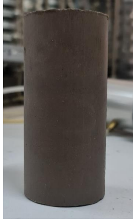
Figure 5.2: Samples reinforced by 3%, 5%, and 10% cement
