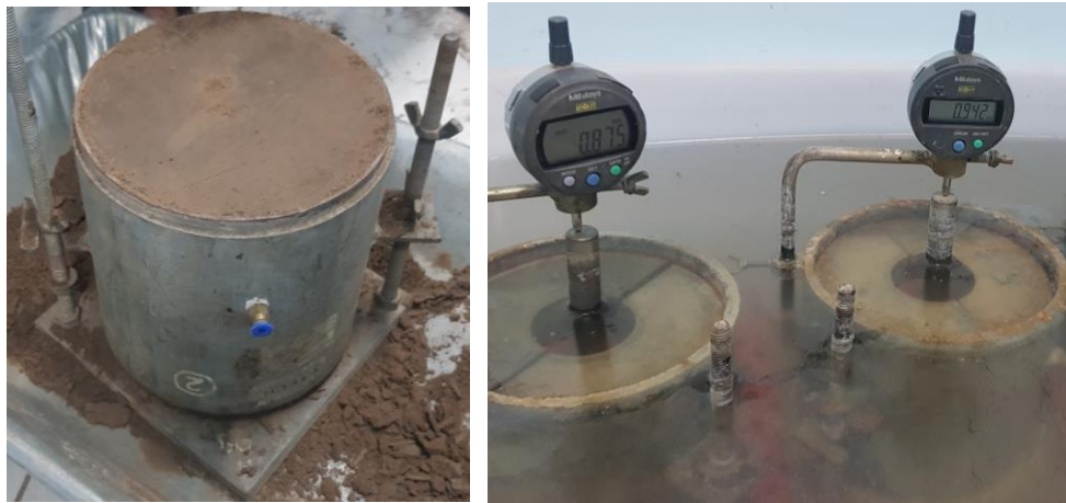
Figure 5.1: Soil cement CBR specimens with 3%, 5%, and 10% cement ratios.
