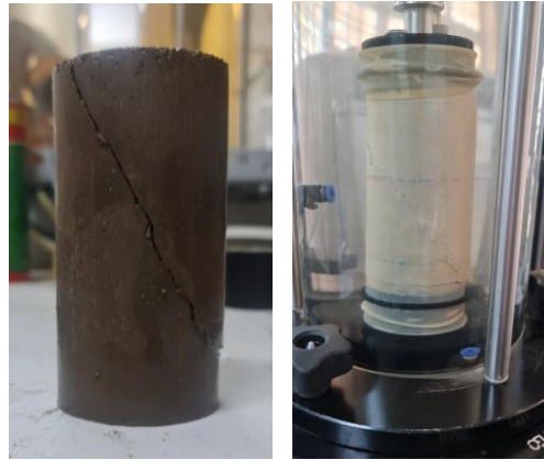
Figure 5.9: The cemented soil samples at failure
