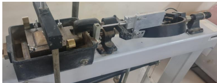
Figure 2.12: Modified shear box for interface shear strength
